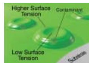
Contaminants can cause surface tension gradients, resulting in a "cratering" or "fish eye" effect.
